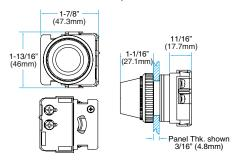
RESISTOR PILOT LIGHT OPERATOR (SHOWN WITH PLL AND IP20 TERMINAL GUARD)
