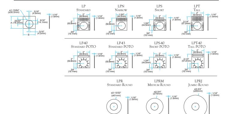
Note: Legend plates feature a tab for optional break-away positioning and can be used in conjunction with the Thrust & Trim Washer accessory.
