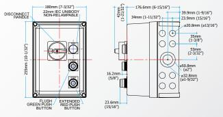
Enclosure Type "H" (Shown with MPCB, Contactor, Disconnect Switch, Pilot Light and Selector Switch)
