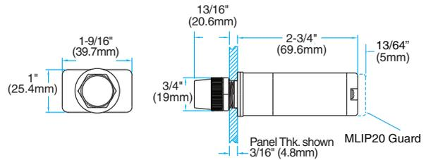
Multi-Voltage Pilot Light/120V & 125V Resistor Indicating Light
