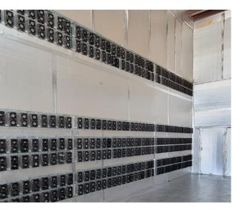
"In layman's terms, ASIC mining is simply special built computers to run hash functions," says Staggs. "A typical unit is about 18 inches by 12 inches by 10 inches, and uses around 3,100 watts of consistent power, which would be similar to running a household electric clothes dryer." Staggs explains that operating his 113 100-terahash ASIC units at Peake Holdings is like running 113 electric dryers 24/7/365 – only profitably.
