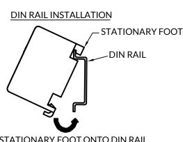
LATCH STATIONARY FOOT ONTO DIN RAIL, THEN ROTATE THE TERMINAL BLOCK UNTIL THE BOTTOM FOOT ENGAGES
