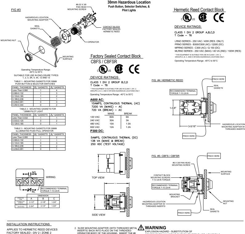
BEFORE INSTALLING THE OPERATOR TO THE 1 PANEL, REMOVE THE OPERATOR MOUNTING NUT AND SLIDE THE SEAL GASKETS AND THE MOUNTING ADAPTER BACK EXPOSING THE BOTTOM OF THE OPERATOR HOUSING. SNAP THE CONTACT BLOCK ONTO THE OPERATOR HOUSING. A DISCERNABLE "CLICK"- IS HEARD WHEN THE CONTACT BLOCK IS SNAPPED IN.
