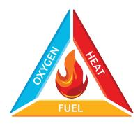
These three elements form the "Ignition Triangle." Removing any one of them prevents an explosion.
