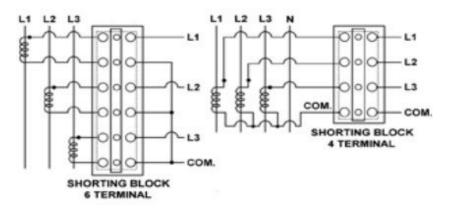
The choice between four-pole and six-pole shorting blocks often depends on the specific requirements of the electrical system and the need for maintenance access.
