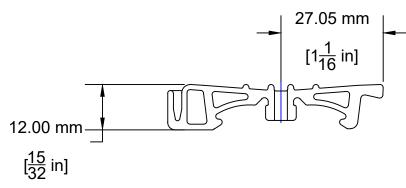
RECOMMENDED SCREW FOR INSTALLATION OF MOUNTING CLIP IS M4 (#8) SELF TAPPING SCREW
